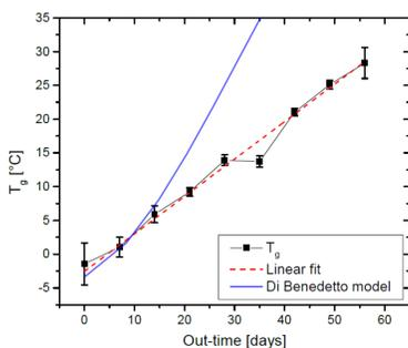
The DSC can be used to work out the out-time from the  $T_g$ .
