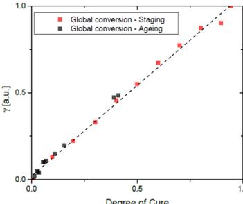
Successfully recorded the evolution of prepreg's state while ageing and staging recording the conversion of functional groups typically involved in the cure of epoxy as:
