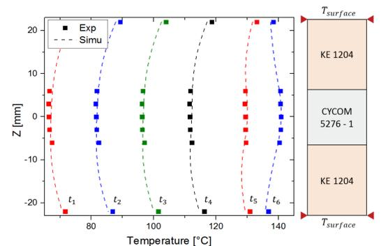
Good agreements between the experimental and simulated thermal profile, the cure kinetic model of the resin is then validated and can be used to simulate the evolution of the degree of cure while staging
