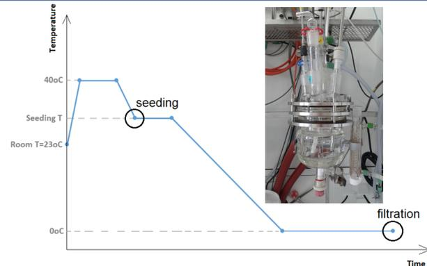
The generic temperature versus time profile of crystallization experiments and the 1L reactor that was used.
