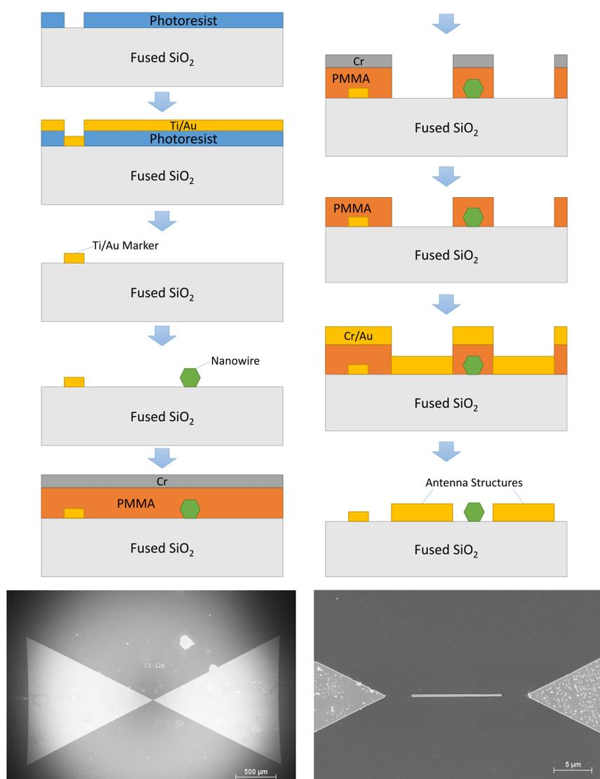
Figure 1: Process flow for antenna fabrication and resulting SEM images of one device.
