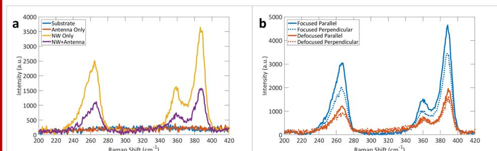
Figure 2: a) Raman spectra for fused silica substrate, reference antenna with no nanowire, GaAs/AlGaAs nanowire with no antenna and similar nanowire with antenna. b) Focused and defocused polarization-dependent Raman spectra.
