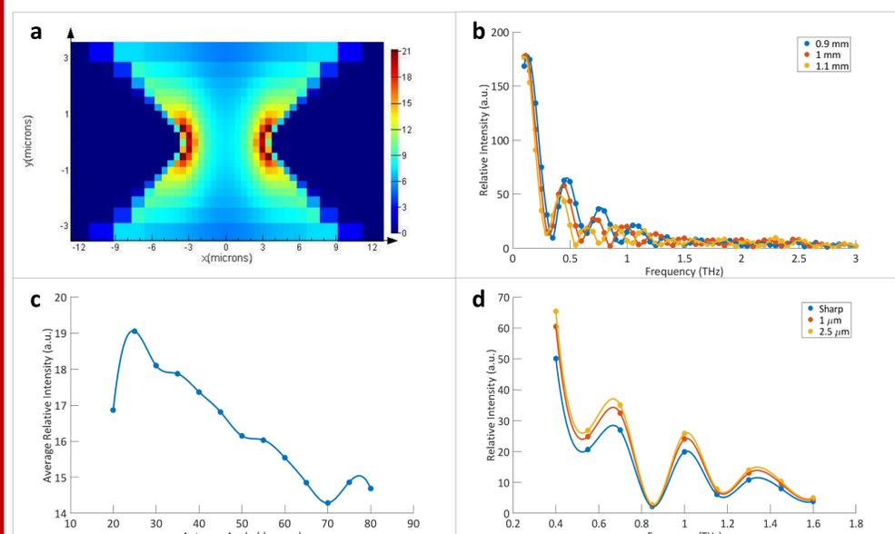
Figure 3: a) Spatial map of field enhancement at antenna tip for a frequency of 1 THz. b) Field enhancement as a function of frequency for three antenna sizes. c) Average field enhancement from 0.4 – 1.6 THz as a function of antenna angle. d) Field enhancement as a function of frequency for sharp and rounded antenna tips. Legend gives radius of curvature at tip.
