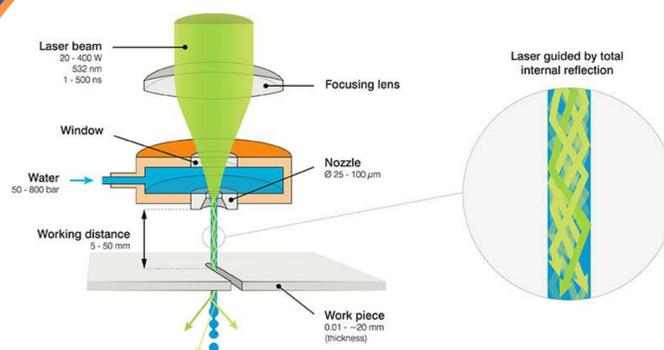
The Laser Microjet® technology focuses a nanosecond pulsed green laser in a micro-metric diameter water jet. The water jet is guiding laser light through thick samples allowing fast cutting. The water jet is cooling the material, removing burrs and debris resulting in high-end cut quality and precision.
