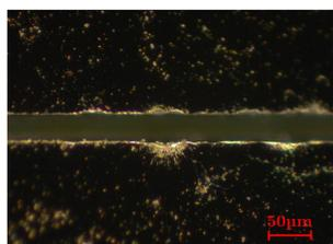
Jet instabilities were reduced using a low water pressure, low power laser parameters and a high cutting speed. Thus limiting splashes.
