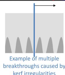
As the last layer of material is being cut, the force applied by the jet and the shockwaves created by the pulsed laser cutting both induce stresses fracturing the material, creating a chip. After breakthrough, the jet is tangent to the cutting surface and stresses do not cause more chipping. However if the cut is irregular breakthrough will occur multiple times creating several chips. Thus stable ablation is critical in order to avoid creating backside chipping.
