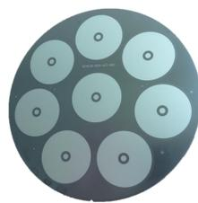
Downsizing of 8 circular pieces in silicon wafers with three thicknesses: 175µm, 420µm and 1450µm. The application required limitation of heat damages and backside chipping smaller than 50µm.
